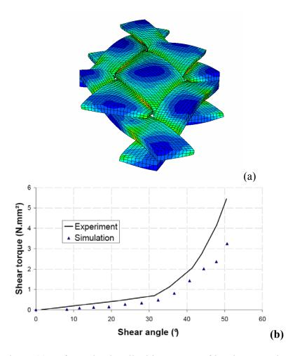
Fig. 3 (a) Deformed unit cell with contours of local compaction; (b) Shear curve, simulation vs experiment.
